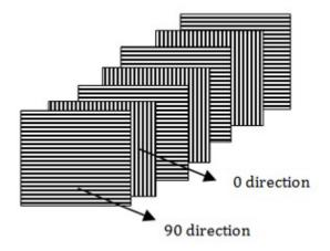
Fig.3. Layered arrangement
