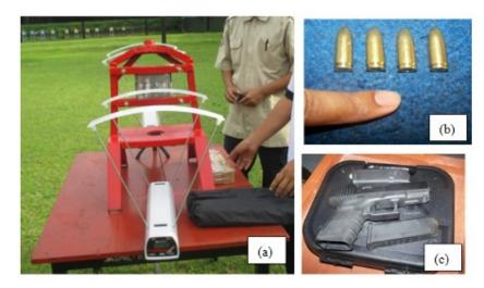
**Fig.8.** Ballistic test setting (a) RFRE composite which able to withstand the projectile (b) Projectile (c) Magnum gun
