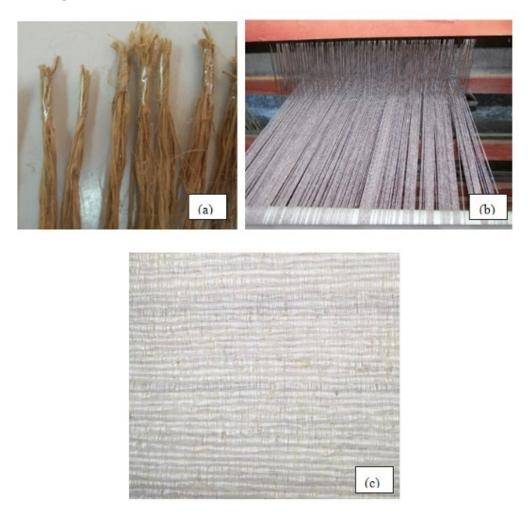
**Fig.2.** Processing ramie fibers to be composite reinforcement (a) ramie fibers cutting process (b) cotton yarn (c) woven ramie fiber (lamina)
